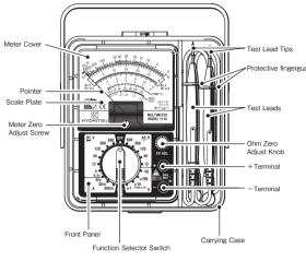
Protective fingerguard:It is a part providing protection against electrical shock and ensuring the minimum required air and creepage distances. Caution:Keep your fingers and hands behind the Protective fingerguard during
